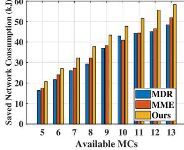
Fig. 12. Saved network consumption vs. Available MCs in test-bed experiments.
