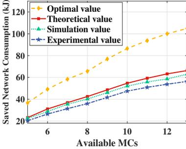
Fig. 11. Comparison among theoretical results, simulation results, and experimental results.
