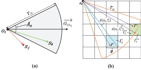
Fig. 2. (a) Charging model: SC can only charge the sensors within its sector charging area (e.g.,  $s_k$ ) rather than outside sensors (e.g.,  $s_j$ ). (b) Area discretization.
