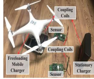
Fig. 9. Test-bed in realistic scenario: SC, freeloading MC, and sensors.
