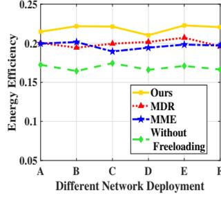
Fig. 8. Network energy efficiency: Freeloading vs. Without freeloading.
