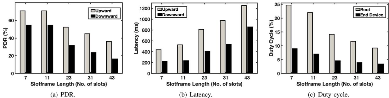
Fig. 4. Performance when the network uses different slotframe lengths.
