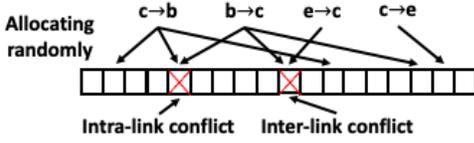
Fig. 7. Example slot conflicts. A slotframe consists of 18 slots. The numbers of cells scheduled for link  $c \rightarrow b$ ,  $b \rightarrow c$ ,  $e \rightarrow c$ , and  $c \rightarrow e$  are three, three, one, and one, respectively.
