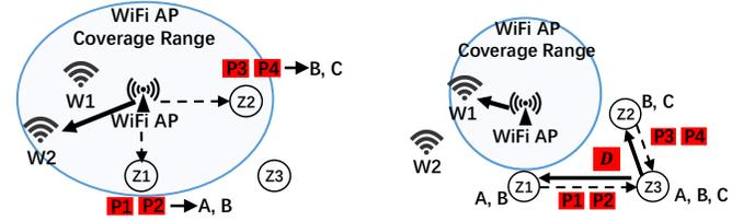
(a) Z1 and Z2 receive insufficient number of coded packets from WiFi AP. Each node can only decode two packets. (b) Z3 has received enough packets and can decode A, B and C. Then, it can broadcast one coded packet D to Z1 and Z2.
