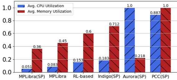
Fig. 17: The normalized overhead comparisons of learning-based methods. The schemes that are marked with "SP" are single-path methods.
