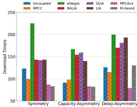
Fig. 15: The download time comparisons of a 75MB file through symmetry and asymmetry networks.
