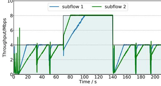
Fig. 3: Illustration of throughput variations for LIA with two subpaths, where the capacities of two links increase from 4 to 8 Mbps at 70s and decrease from 8 to 4 Mbps at 140s.
