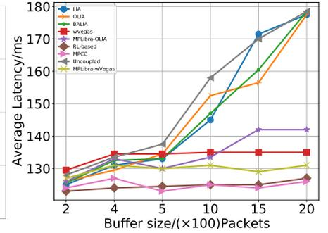
Fig. 16: Average latency under different buffer sizes
