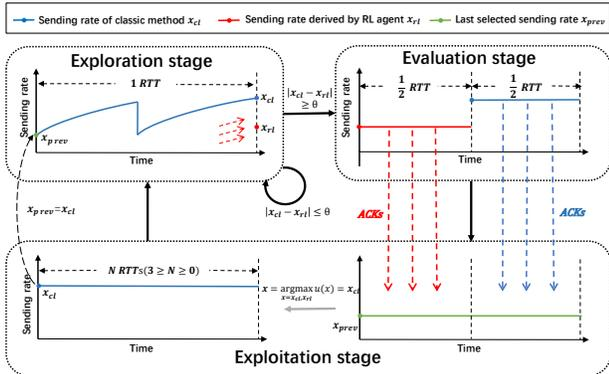
Fig. 6: Time-diagram of the Stage Manage Module in Fig.5
